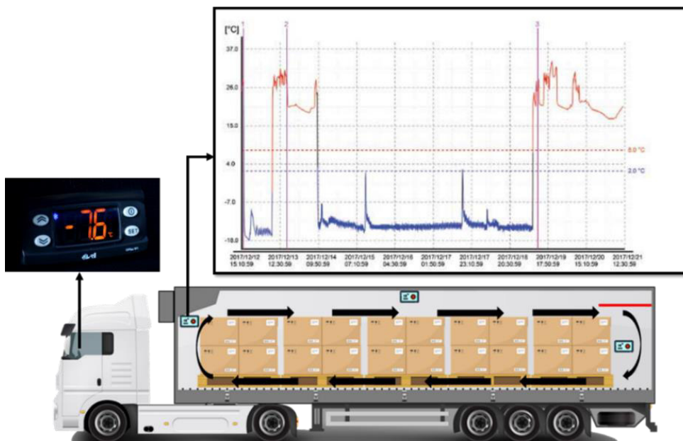
Figure 4.8 Refrigerated truck and temperature monitoring graph
