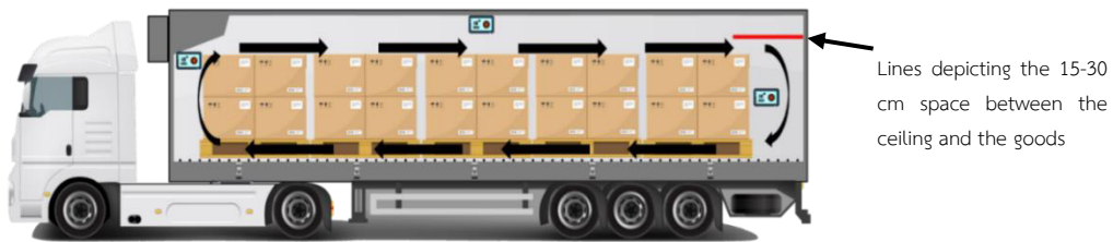
Figure 4.7 Product placement in a refrigerated chamber
