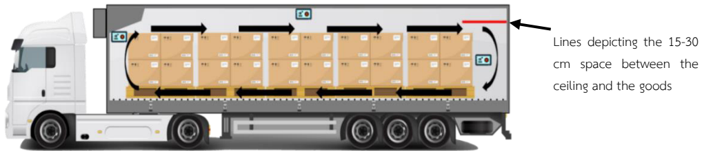
Figure 4.7 Product placement in a refrigerated chamber
